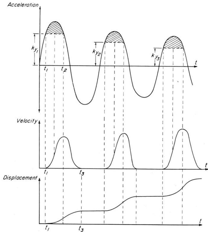
FIG. 8.—INTEGRATION OF ACCELEROGRAMS TO DETERMINE DOWNSLOPE DISPLACEMENTS
